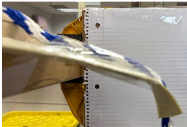
Figure 6.1.2.2: Fin Tip Loaded with 14 lbf, Tip Showing Signs of Significant Failure In Original Design
