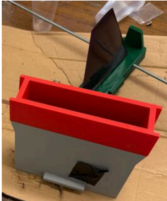
Figure 3.5.2.1: Solid Mold Casting Box (Bottom) And 3D Printed Fin Positive (Purple/Top) Affixed To Casting Sled (Green/Top)
